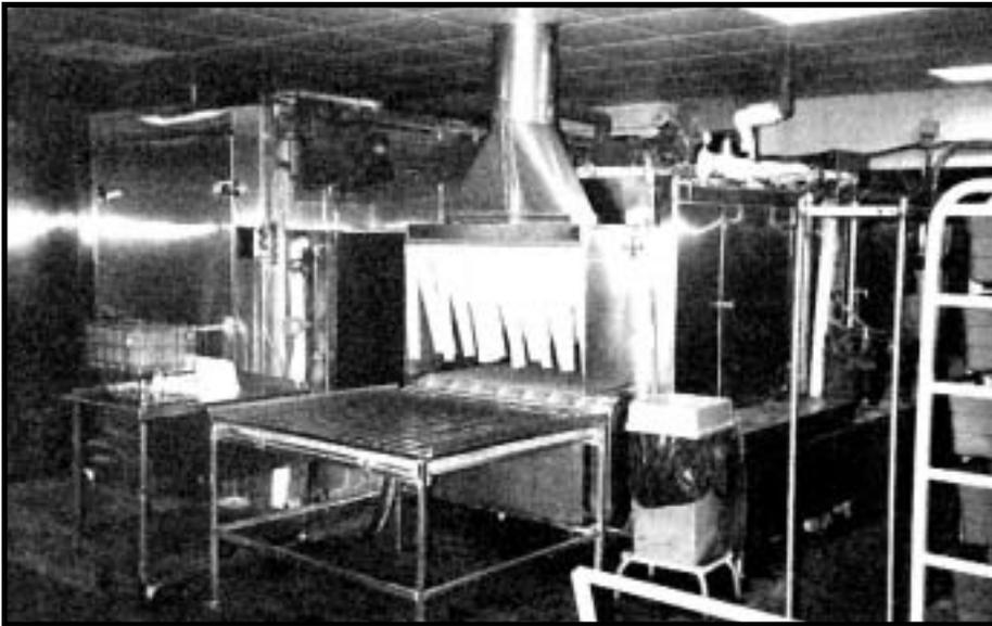
*One of three automated cage washing systems. Works 12 hours per day at 180°F.*
