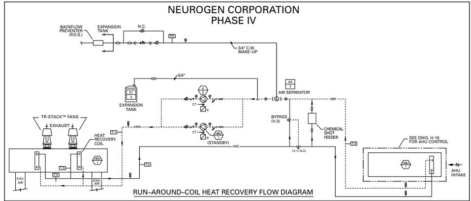
▲ **The Neurogen heat recovery system is energized through the ATC system based upon outside air temperature (OAT). When OAT is below 45° F or above 80° F, the heat recovery supply valve (V1) opens, the bypass valve (V2) remains closed and the pump is turned on. This unique system pre-heats makeup air for the intake ventilation system at least 10°F, resulting in a 30% reduction in heating costs. Built-in safety features prevent heat loss in case of equipment malfunction.**
