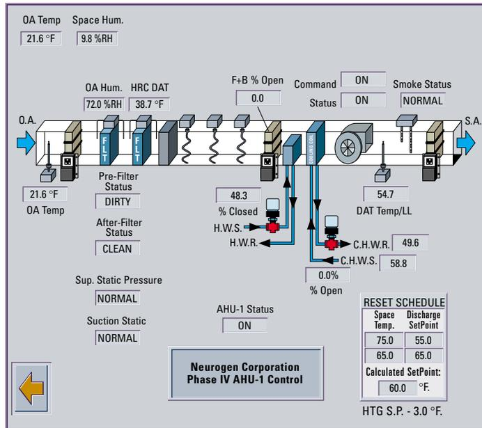
▲ **System status screens such as this provide real time data on system operating and performance parameters. The difference between the indicated outside air temperature and the air temperature after it passes through the heat recovery coil represents energy savings.**
