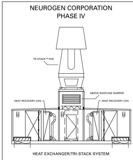
▲ **The exhaust air heat recovery module at Neurogen Corp. is composed of Tri-Stack laboratory workstation fume exhaust systems with accessory glycol/water heat recovery coils inside stainless steel casings. The fan/heat exchanger package pre-heats or pre-cools building intake air at Neurogen's conditioned 100% makeup air Phase IV facility. Dampers above the roofline help provide constant air volume to maintain discharge velocity.**
