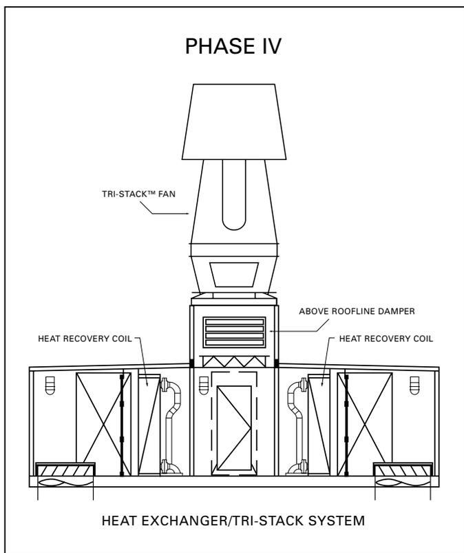
Figure 4. Heat exchanger/mixed flow exhaust system.
