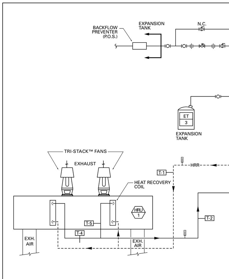
Figure 5. Run-around-coil heat exchanger recovery flow diagram.
