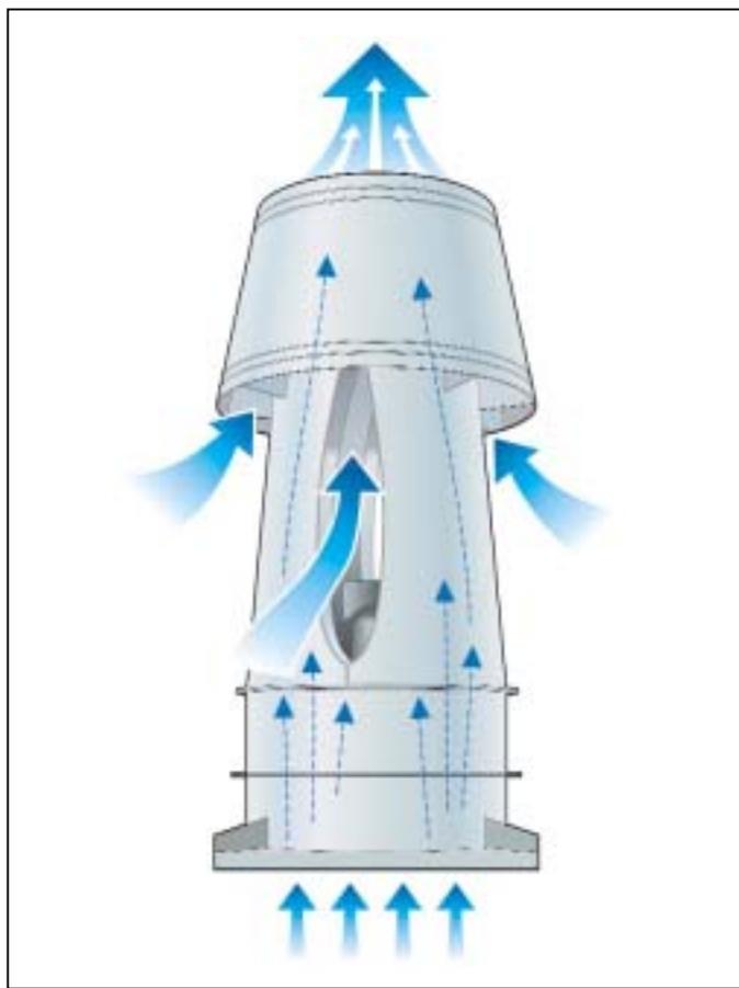
Figure 6. Typical mixed flow impeller system.
