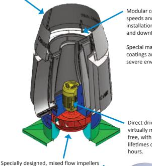
Specially designed, mixed flow impellers provide high pressure and volume at low RPM and mount directly to motor shaft without belts or pulleys. Modular construction speeds and simplifies installation, reduces cost and downtime.
